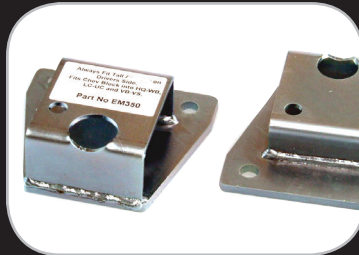
EM350 - Allows Chevrolet V8 to be fitted into HQ-WB Holden, LC-UC Torana & Commodore VB-VS
