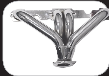
40500 - Fits SB Chevy 265-400. Fits regular or slant plug heads [8mm flange & reducer] Tube diameter 1 11/16" with 3/32" thick material. Includes collector reducers, gaskets & header bolts. Chrome Finish 40501 - As above, Black Finish
