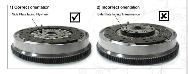
2. If converting an Automatic to Manual transmission be sure to have the flywheel professionally re-dowelled to suit the Automatic Engine Crank. Failure to do so may cause unwanted vibration due to off centre mounting of the flywheel.
