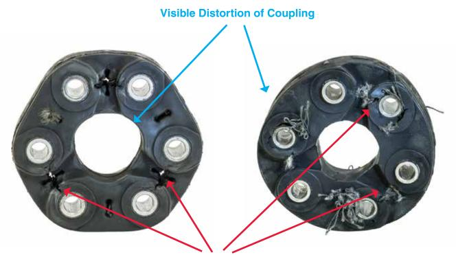
Torn rubber in thin section shows signs that it has taken drive load.
